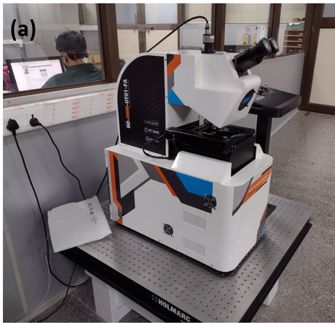
Figure 1. Digital holographic microscope system used in the present study. (a) System photograph. (b) Nominal optical layout of the system. B_1, B_2, B_3 : beam-splitters; M : plane mirror. The beam-splitter B_3 can be rotated with an adjustable screw in order to introduce tilt in the reference wave as required for off-axis hologram recording. The system is fitted with a laser source for phase imaging and LED illumination with condenser for bright-field illumination. By switching between the two illuminations, one can record an image plane digital hologram or a bright-field image of the sample in the same position.
